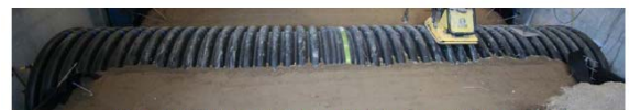
c. 1500 mm (60 in.) diameter high density polyethylene pipe with bell and spigot joint
