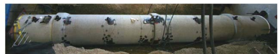
a. 600 mm (24 in.) diameter reinforced concrete pipe with gasketed bell and spigot joint
