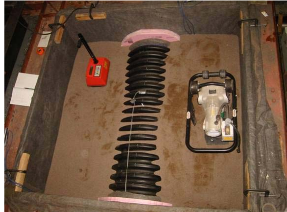
Pipe being installed in the biaxial pipe test cell at Queen's University
