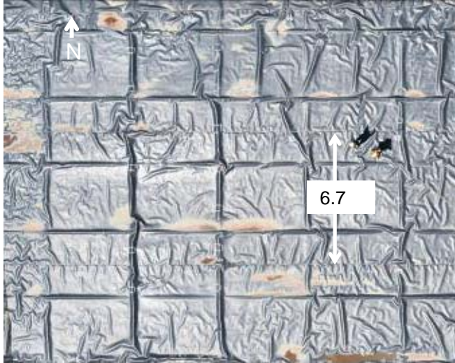
Figure 12 Aerial photo showing a small portion of connected wrinkle network on the base liner at QUELTS (same bottom liner as shown in Figures 8 and 11) Taken on 28 May 2008 at 1:00pm; air temperature of 11°C; GM temperature on the base of 53°C. Distance between GM seams is approximately 6.7 m as shown. Modified from Rowe et al. (2011b).
