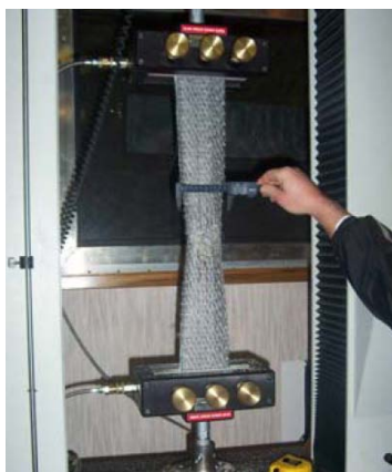
Figure 4. Example of laboratory tension-necking test. (courtesy of Koerner and Koerner 2005a)
