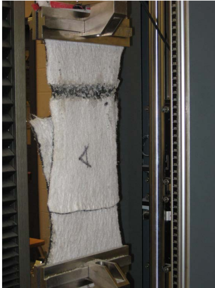
Figure 9. Tensile failure of specimen by pre-engineered groove.
