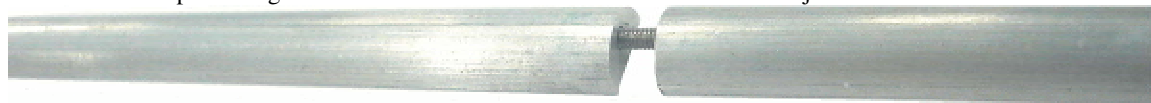
b. A larger view of two segments of aluminum half-pipe and the steel rod representing the joint.
