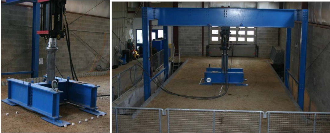
a. Close-up of load frame
