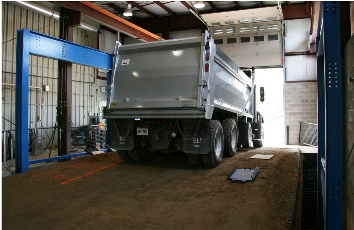
Figure 5. Truck over the culvert during testing.
