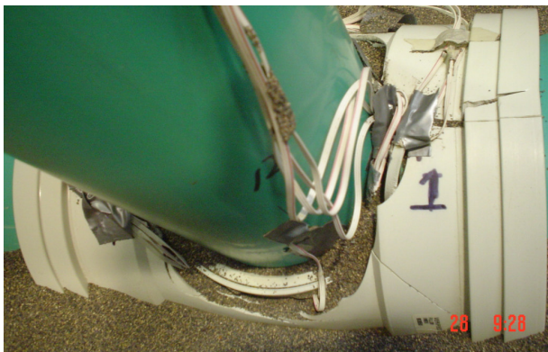
Figure 14. Fractured Tee fitting in sand
