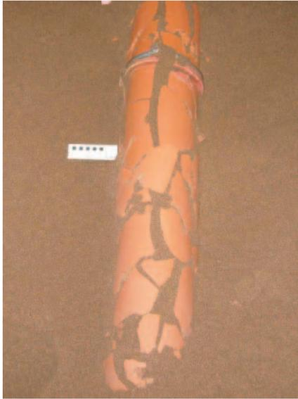
**Fig. 7.** Fracture conditions, Test 2.
