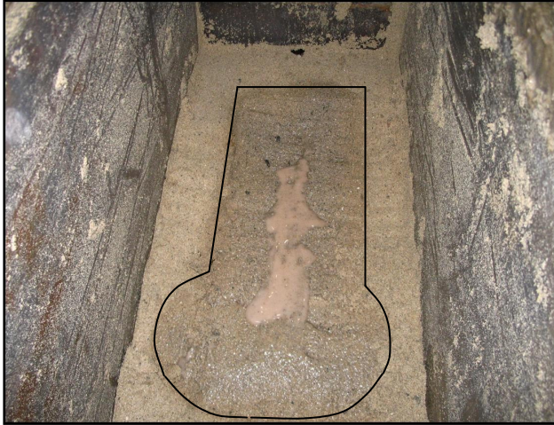
Figure 2 – Filtercake at the borehole crown
