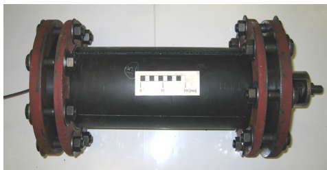
a. Laboratory test specimen b. Internal pipe restraint
