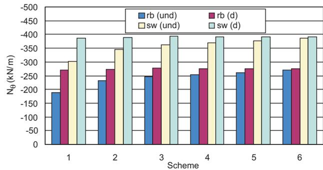
**Fig. 12.** Maximum shear forces in the wall and hopper. d, drained; und, undrained.
