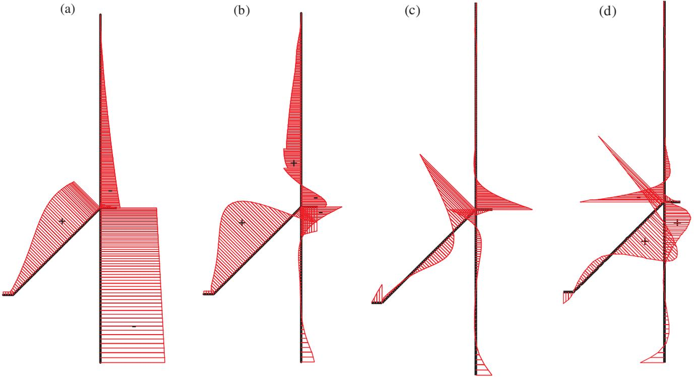
**Fig. 8.** Maximum axial forces due to different filling schemes in the wall and hopper. d, drained; und, undrained.
