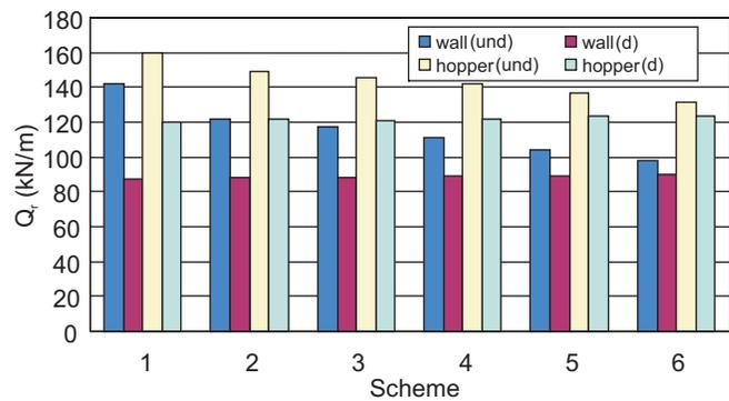
**Fig. 13.** Maximum bending moments in the wall and hopper. d, drained; und, undrained.
