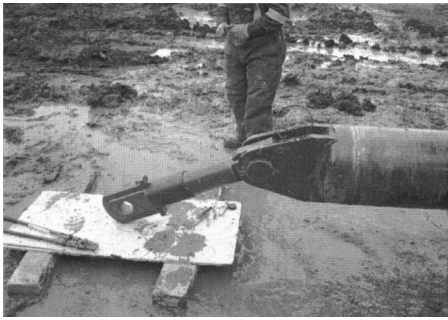
Fig. 1. 670 kN capacity loadcell attached to 406 mm diameter pullhead
