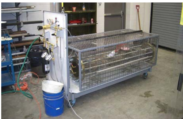
Figure 6. Custom-made pressure cell - 12 equality-space high-strength threaded rods are used to apply a compressive force to the ends of the specimen.
