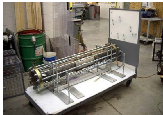
Figure 6. Custom-made pressure cell - 12 equality-space high-strength threaded rods are used to apply a compressive force to the ends of the specimen.
