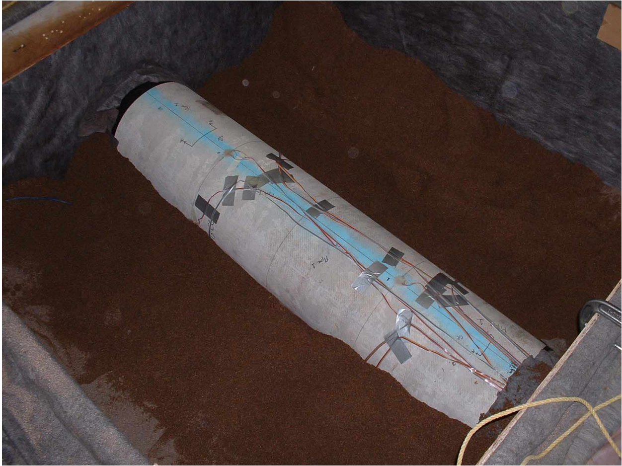
Figure 4. Dry pipe specimen being buried in the test cell; image shows geosynthetic used to protect sidewall friction treatment.
