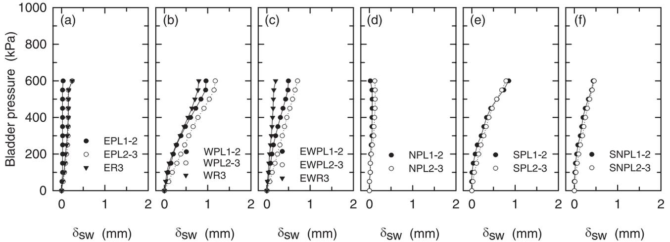
**Fig. 13.** Lateral deflections of the exterior walls of the test cell measured during test T3: (a) east wall; (b) west wall; (c) average of east and west walls; (d) north wall; (e) south wall; (f) average of north and south walls.
