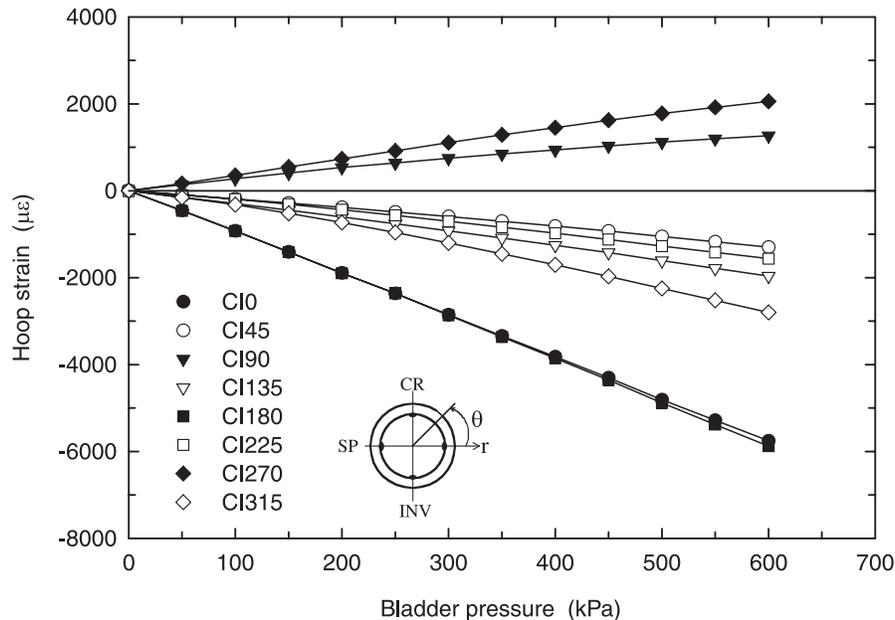
values. The reported values of strain versus applied bladder pressure represent the strain averaged over the last 30 s of each 40 min pressure increment. Each pressure step involved the rapid application of an incremental bladder pressure of 50 kPa, which was then held constant for the duration of the pressure step.
