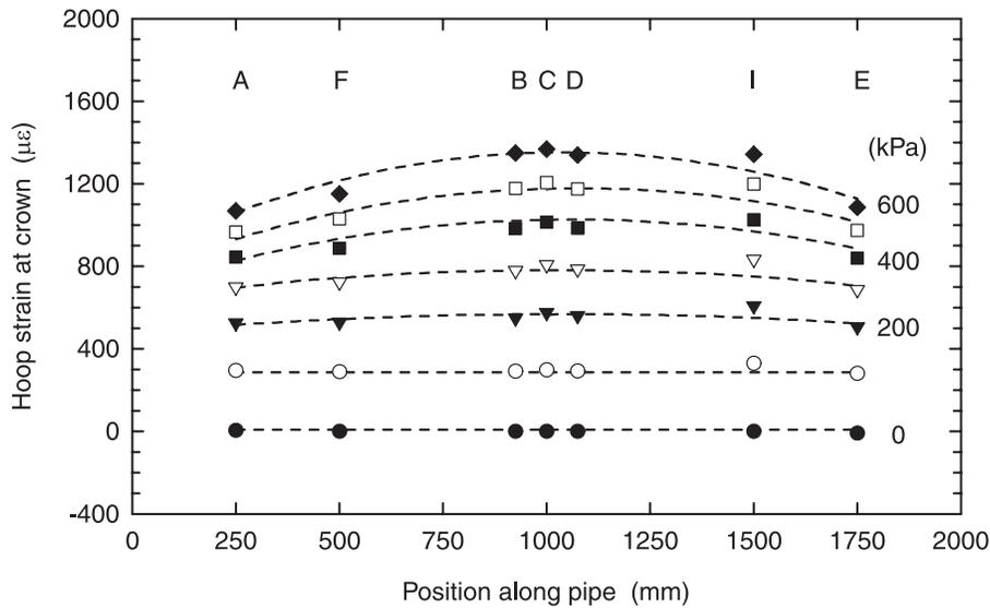
Fig. 9. Variation of hoop strain measured at the interior springline location along the pipe during test T1.
